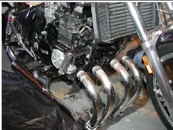
**#16** At this stage, the assembled exhaust system rests on the floor with the collector ahead of the centre stand and the downpipes just behind the front wheel. Therefore, to move the exhaust system clear of the bike, it has to move both forward and to either the left or right side. As you push it forward, swing the downpipes out a bit farther, in this case to the right of the bike, for which it may help to turn the wheel fully to the right as well.
