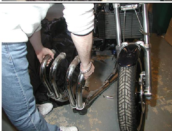
**#18** The end result - the exhaust system stayed in one piece and was successfully removed with the bike on the centre stand and by one person with only minimal help from an assistant.
