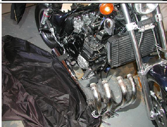
**#17** When the downpipes are past the front wheel and out to the side of the bike, just take hold of the outer two downpipes to lift and pull the assembled exhaust system fully away from the bike.
